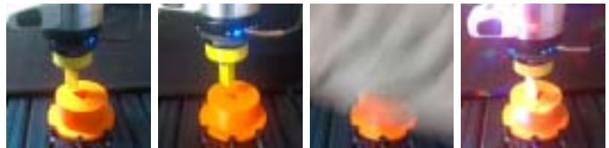
Fig. 11: Visual disturbances of the robustness evaluation. From left to right: back light, front light, occlusion, and disco lights. MSDP achieves a high success rate across all disturbances, which have not been seen during training.
